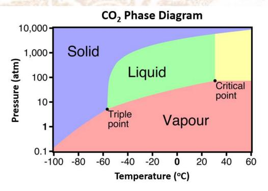
It should be noted in looking at the diagram that in many sequestration projects, the phase of CO<sub>2</sub> will be in the "yellow" area of the graph. This is the super-critical phase.
