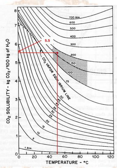
From the chart above it can be seen that the solubility of  $CO_2$  is 5.5 kg/100 kg, which equals 5.5 lb/100 lb water at sequestration conditions at a pressure of 165 bars and 50°C.
