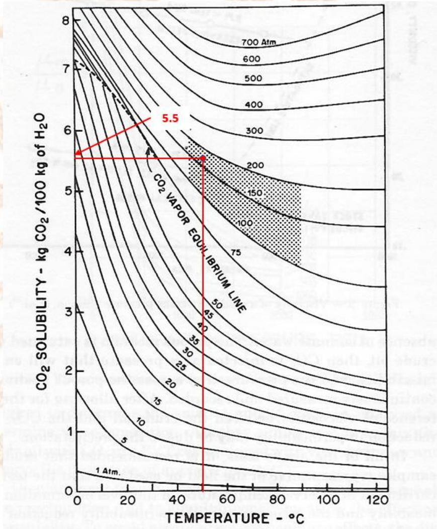
From the chart above it can be seen that the solubility of CO<sub>2</sub> is 5.5 kg/100 kg, which equals 5.5 lb/100 lb water at sequestration conditions at a pressure of 165 bars and 50°C.
